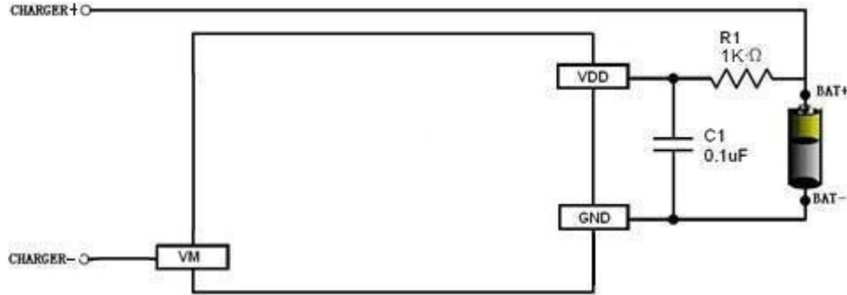
**Fig 6 HY2150A in a Typical Battery Protection Circuit**
