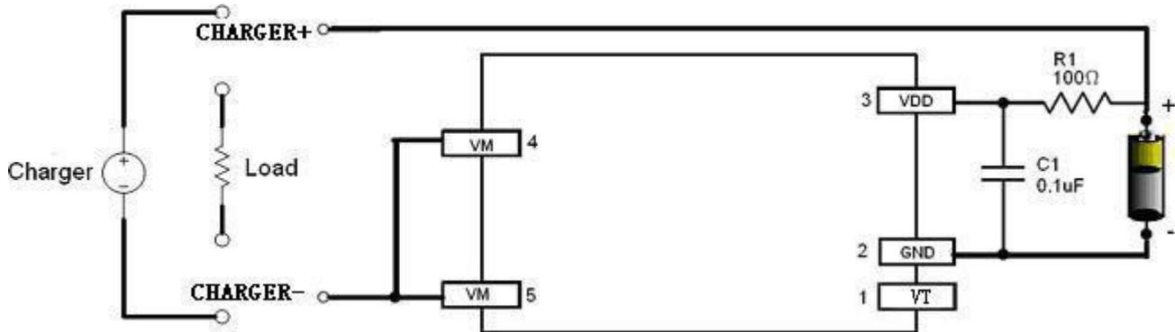
Fig 6 HY2130A in a Typical Battery Protection Circuit
